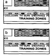
right of the lit indicators is flashing (see drawing a), increase your pace. If an indicator to the *left* of any lit indicator is flashing (see drawing b), decrease your pace. When no indicator is flashing, your heart rate is near the current heart rate setting. Important: The heart rate settings are intended only to provide motivation. Your actual heart rate may be slower than the current heart rate setting. Make sure to exercise at a pace that is comfortable for you.
